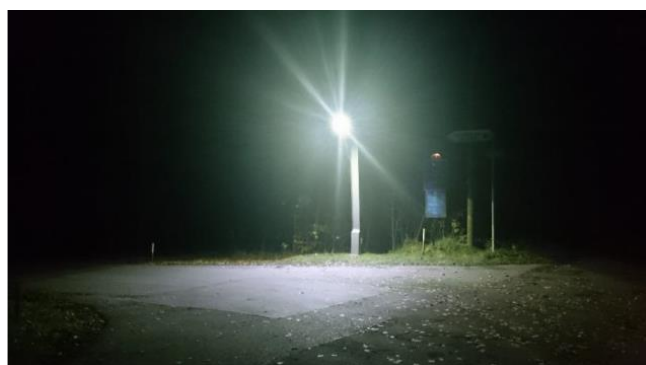
100% light intensity after activating movement sensor (adjustable)
